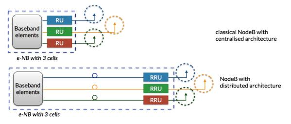
Figure 1. A classical compact BTS/a centralized architecture and a Distributed Architecture
