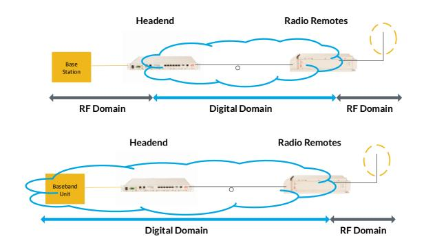
Figure 4. The RF Router system interfaces with the base station via an RF interface or directly to a digital baseband interface (BBI).
