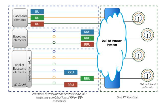
Figure 7. Dali's RF Router can deliver immediate benefits to an operator without a major overhaul to their network. It works with existing centralized architecture, distributed architecture and C-RAN.
